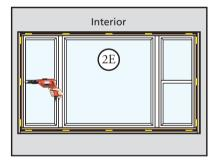
F. If desired, shim and fasten headboard to rough opening. To keep plywood straight, center one finish head screw or 10D finish nail on units less than 10 feet wide and equally space two fasteners on units wider than 10 feet.
